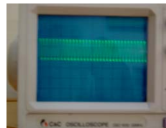
Offset/DC Level in AC Signal
